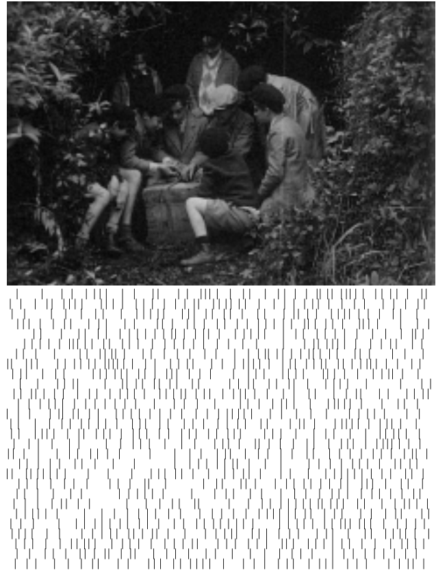
Figure 2: Telecine example (720x576) showing a small scratch (in fact, only visible in the blue plane) and corresponding raw, untracked, detection using 16 pixel-height projected stripes
